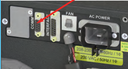
Modbus RTU Communications Model: 485 or 232-MODBUS RTU
